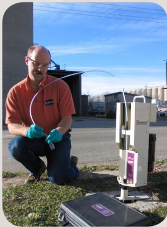
The Geoprobe® Electric Actuator, in combination with the Mechanical Bladder Pump (MBP), allows for the collection of high quality, low turbidity groundwater samples from direct push installed small diameter groundwater samplers and monitoring wells. The 12-volt Electric Actuator minimizes the field effort to conduct low flow sampling by electrically completing the sample retrieval process instead of the field operator doing it manually.
