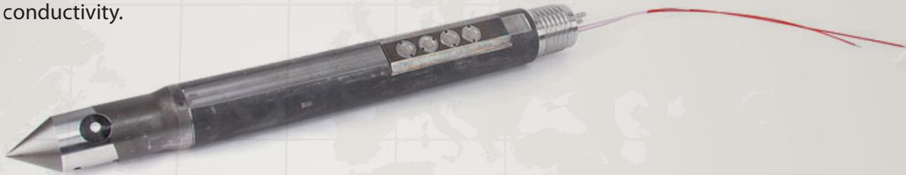
The HPT log of this tool serves the additional purpose of indicating zones that are appropriate (exhibit sufficient permeability) for groundwater sampling. The operator can stop advancement of the tool in these zones and switch to groundwater sampling mode.
