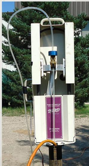
Groundwater samples are pumped to the surface using a Geoprobe® Mechanical Bladder Pump (MBP) incorporated into the top of the HPT-GW Sampler. A ¼ inch (6.4mm) OD Teflon® tube is commonly used as the sample flow line from the pump to ground surface. Typical flow rate during groundwater sampling with this tool is 200 ml/min. However this rate can be varied from 25 to 300 ml/min by adjusting the speed of the pump electric actuator.
