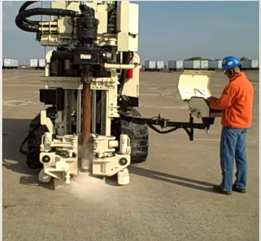
Geoprobe® model 8040DT running the GH80 Concrete Breaker System through 10 in. of concrete.
